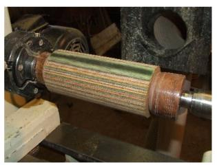
I have mounted the body of the mill on specially made jam chucks. The bottom of the mill is towards the tail stock, but orientation here is the turner's choice. This is my preference... dictated by the fact that this is the way I cut the original jam chucks.
