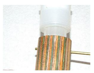
Dry fit the 1/8" brass rod to make sure you have the hole in the correct place and mark it to length for cutting. I generally pull the rod until one end is near flush, then mark the other end as close to the body as possible. The ends of the rod can be sanded smooth on a belt or spindle sander.
