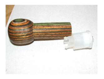
If you have not already, it would be wise to again dry fit the mill parts to make sure the top fits flush and snugly against the mill body.
