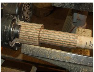
Now turn a tenon on the cap end of the mill to a smooth and uniform size of approximately 1 17/32" diameter. This tenon will need to fit inside the main body of the peppermill and turn smoothly, but not be loose.
