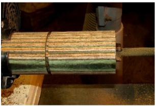
Using the 1 1/16 Forstner bit, drill the cap end of the mill through the blank past the cut line for about 1/2 the distance of the cap. This will be the pepper chamber. The deeper you are able to drill, the greater volume of pepper corns the mill will hold.
