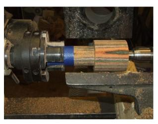
The top chucked into a long nose alligator chuck. I've wrapped the tenon in blue masking tape to keep from marring the surface.
