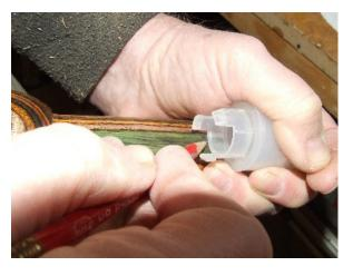
Mark the tenon just above the grinder turning mechanism about 1/8 inch.
