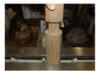
Checking the fit of the top tenon into the body of the mill.
