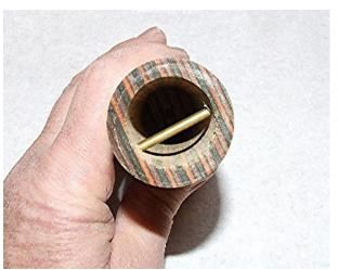
The rod is inserted and has been sanded smooth on both ends. It must be sanded smooth and flush with the wall of the tenon. I use my 1 inch belt sander. The brass will sand quickly and smoothly. You could also use aluminum if you want.
