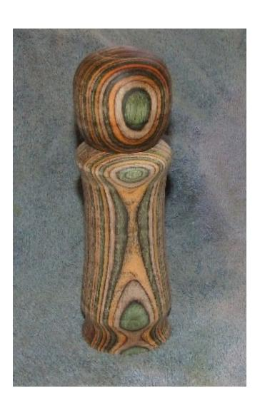
The pepper mill is complete and ready for finishing, using your finish of choice. Final assembly should wait until the finish has cured.
