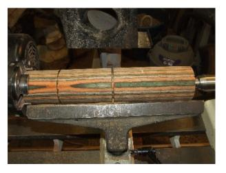
Make initial cuts on the pencil marks and part the blank into two pieces at the center line. The right hand piece will be the body. The left piece will be the top and tenon.
