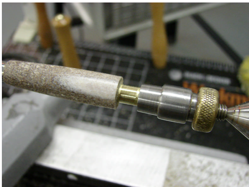
Tenon Cut for Cartridge Head Center Band
