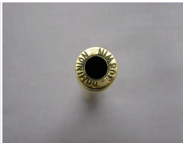
Tube Flush with Bottom Of Cartridge Head
