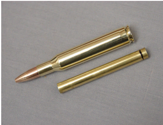
Mark Tube And Cut Flush With Cartridge base
