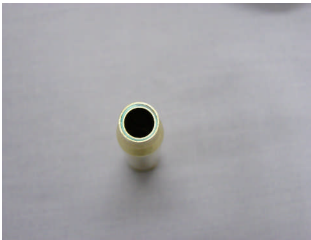
Tube Inserted Into Cartridge Neck
