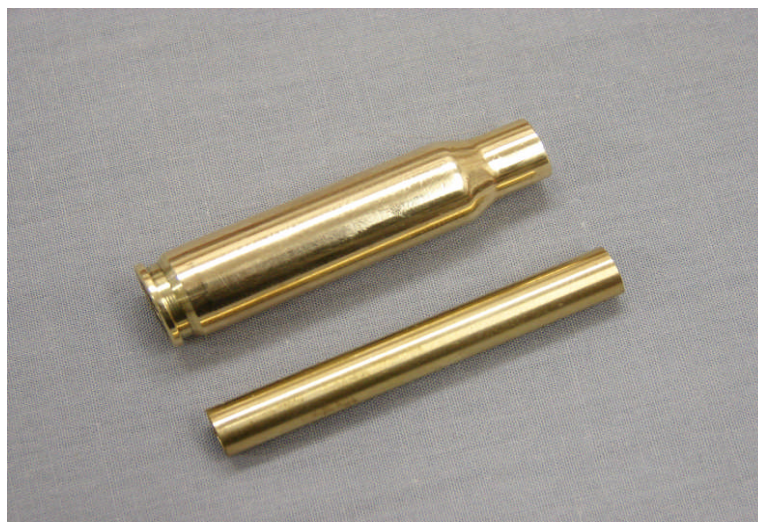
7mm Brass tube cut 1/16” longer than Cartridge
