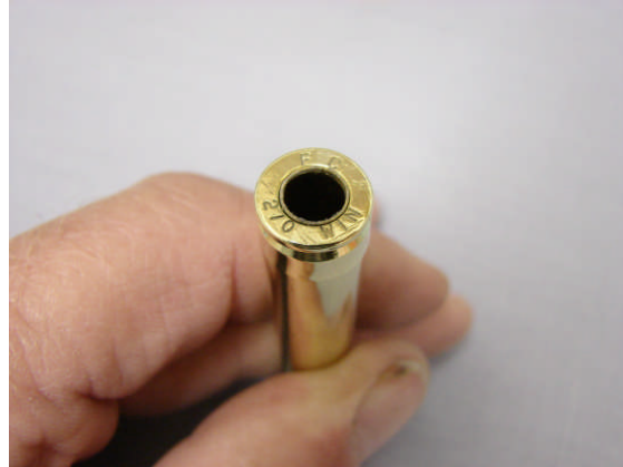
Check Tube Flush With Cartridge Base
