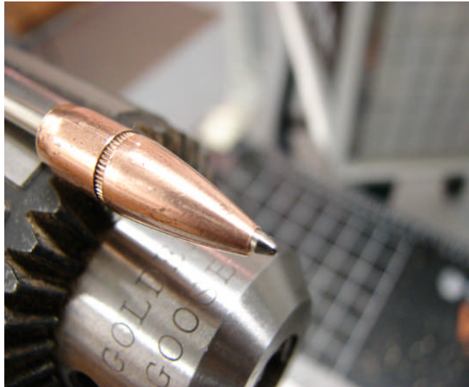
Checking Nib Refill Hole For Reveal
