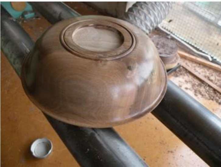
Slightly duller surface from Tripoli abrasive.
