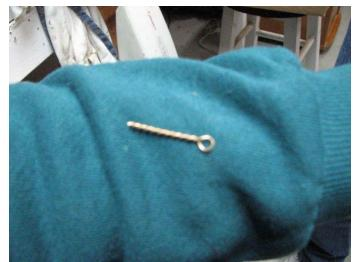
Pull up and twist the wire. You will get a small eyelet hanger. I make these while watching TV and have gotten about 100 or so and haven't even made a dent in the roll of wire. Drill a hole in the top of the cap just so the twisted wire fits in. Put some medium CA glue on the wire and insert in the hole. Let dry for a few minutes. Get your rattle can Lacquer out and give it 2 to 4 coats or more if you want more shine. I put my coats on every 30 minutes using the Deft lacquer.
