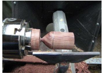
Out of the piece left in the chuck I make a jam chuck to reverse the body on. I use a calipers and mark the size just slightly smaller. Then with a bedan tool, scraper or skew I sneak up on the size where it is a snug fit and won't come off. I then finish the bottom and sand. The body is done for now.
