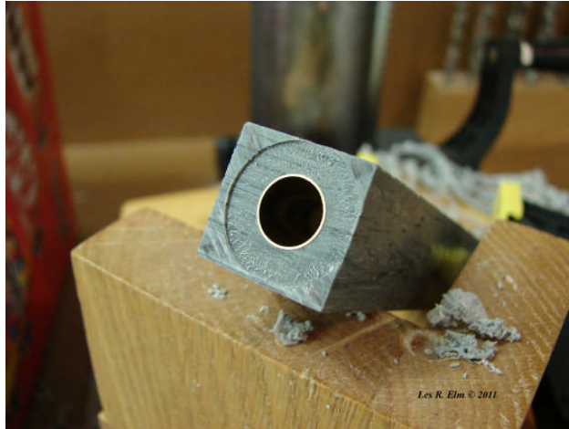
Blank Ends Squared For Total Length of 4-5/16"
