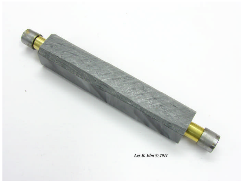
Tubes With Bushing Slide Into the Blank
