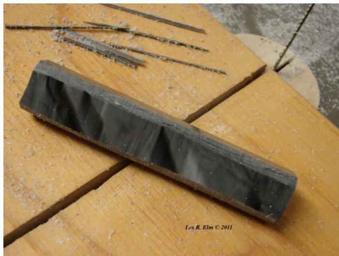
Remove The 4 Corners Off The Blank
