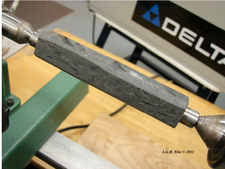
Blank Installed Between Centers c/w Bushings
