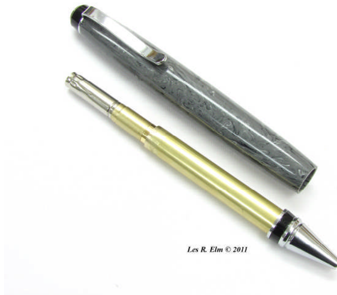
Nib Assembly Ready to Install Into Barrel
