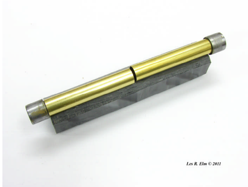
Long Tubes with Cap and Nib Bushings
