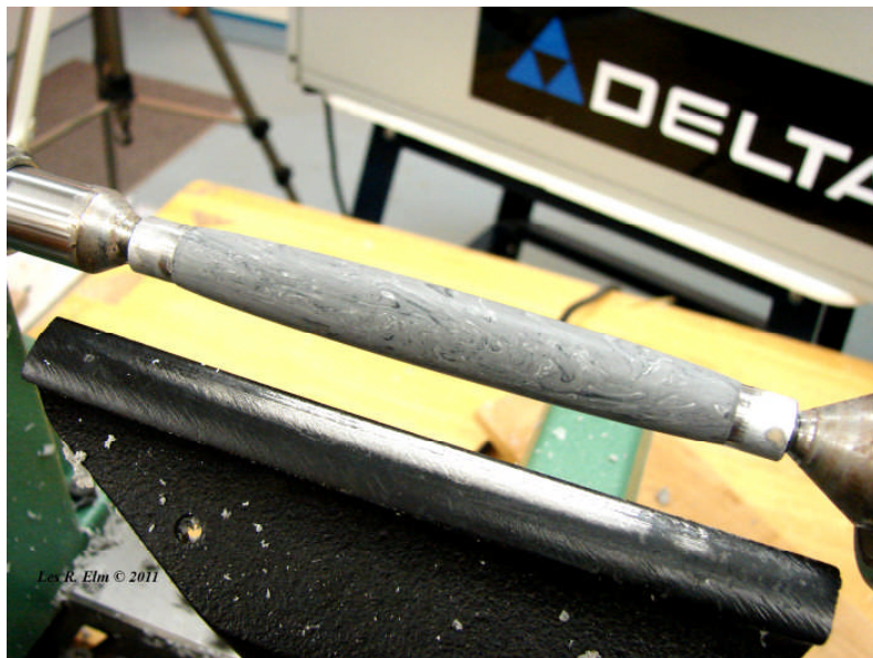
Blank Turned Down and Shaped
