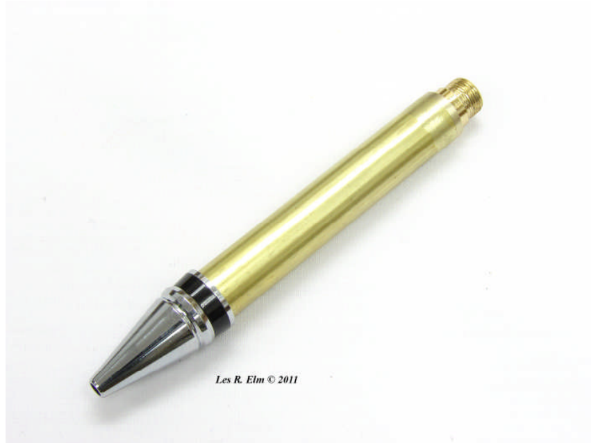
Nib Installed on Lower (Long) Tube
