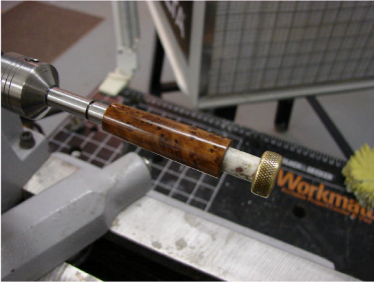
Blank installed on A Mandrel with insert and slim bushings
